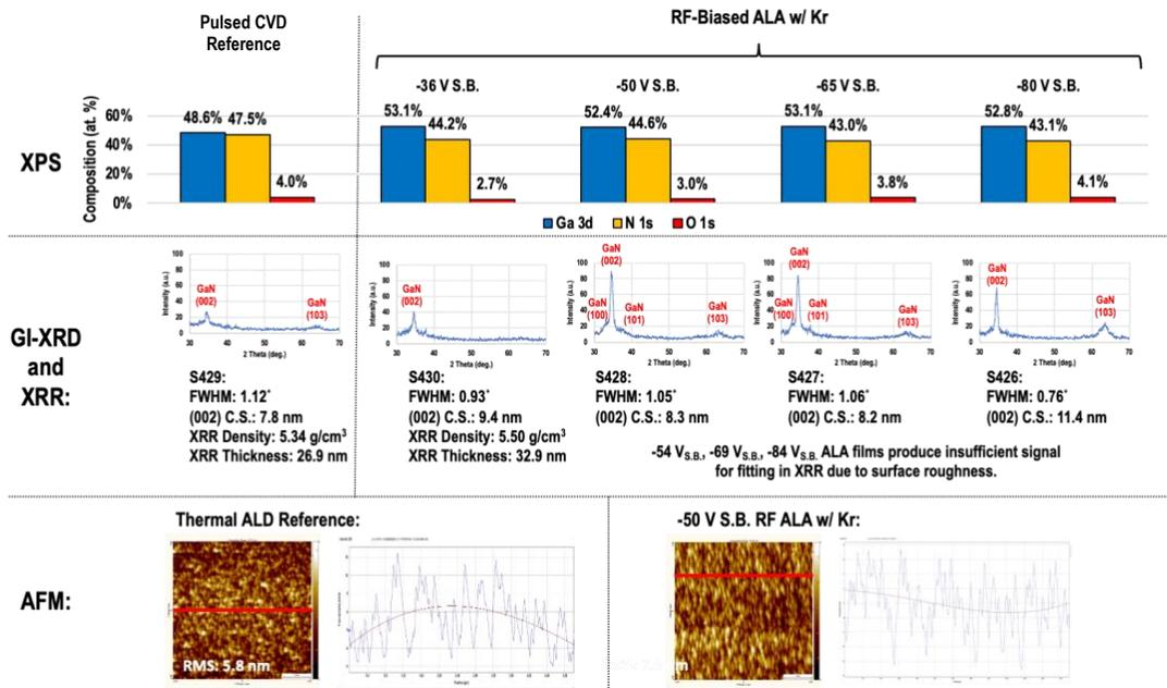
**Figure 2.** X-ray photoelectron spectroscopy composition, grazing incidence x-ray diffraction, x-ray reflectivity, and atomic force microscopy studies of the films deposited by the reference pulsed CVD process and by RF-biased ALA at four self-bias potentials. Note the increased crystallinity due to ALA and increasing magnitude of self-bias potential. Films are roughened by ALA process relative to the pulsed CVD process, likely due to increasing average crystallite size.
