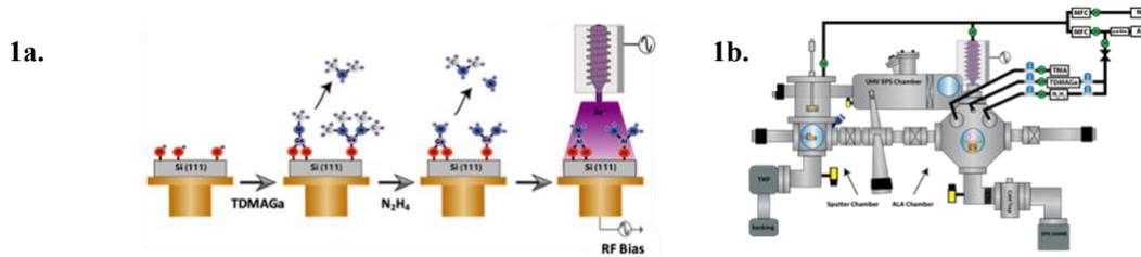
**Figure 1.** ALA process and equipment: **a)** ALA process combines a traditional ALD precursor dosing cycle with a low-energy ion bombardment step at the end of each cycle. This crystallizes the material. **b)** Combination HV deposition chamber, front right, and UHV analytical chamber, back center. Note the chamber allows for XPS analysis without vacuum break by transfer through the load lock chamber.
