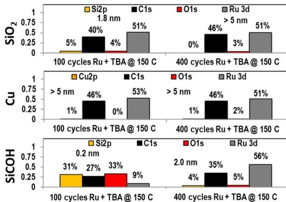
**Fig. 2.** XPS of Ru ALD at 150 °C with Ru(DMBD)(CO)<sub>3</sub> + TBA on SiO<sub>2</sub>/Cu/SiCOH. After the first 100 cycles, SiO<sub>2</sub> and Cu are close to fully attenuated by the overlaying Ru film, while sub-monolayer coverage is present on SiCOH. After an additional 400 cycles, SiCOH is attenuated to ~2 nm Ru coverage while the other substrates are fully buried by the Ru film.
