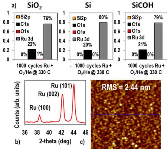
**Fig. 1.** XPS of Ru ALD at 330 °C with Ru(CpEt)<sub>2</sub> + O<sub>2</sub> on SiO<sub>2</sub>/Si/SiCOH. (a) After 1000 cycles, all three substrates fully-attenuated on XPS with O below detection limit. (b) XRD shows distinct peaks for Ru (101), (002), and (100) orientations, with Scherrer approximations showing grain sizes of 25nm. (c) AFM shows film root-mean-square roughness of 2.4nm compared with a film thickness of 52 nm.
