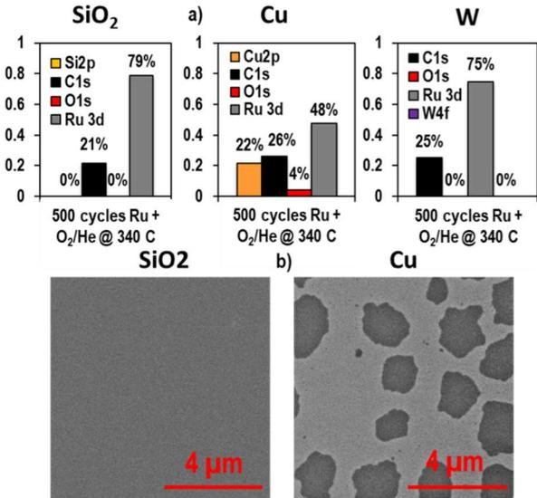
**Fig. 3.** XPS of Ru ALD at 340 °C with Ru(CpEt)<sub>2</sub> + O<sub>2</sub> on SiO<sub>2</sub>/Cu/W. (a)XPS shows full attenuation of the substrates on SiO<sub>2</sub> and W samples, while only partial attenuation on the Cu sample. (b) SEM shows a smooth, uniform film on SiO<sub>2</sub> and W, while on W large voids are observed on the deposited Ru film consistent with the Cu signal observed by XPS.
