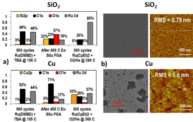
**Fig. 4. XPS of Ru ALD using Ru-DMBD & Ru-CpEt Processes.** (a) XPS of the DMBD process, followed by ex-situ FGA, then CpEt process on SiO<sub>2</sub> and Cu. (b) SEM over a 10x10  $\mu\text{m}$  and AFM over a 2x2  $\mu\text{m}$  area on SiO<sub>2</sub> and Cu after a second ex-situ FGA, showing void formation in the Ru film on Cu and a smooth film on SiO<sub>2</sub>.
