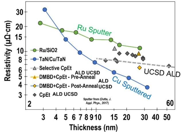
**Fig. 5. Film thickness-resistivity relationship for films deposited via DC sputtering and ALD.**
