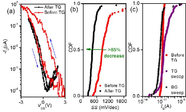
Figure 7. (a)  $I_D$ - $V_{GS}$  characteristics of a 9-AGNR FET before and after (DG sweep) TG fabrication (b) CDF of the SS in 113 devices before and after (DG sweep) TG fabrication. (c) CDF of the  $I_G$  in 113 devices before TG fabrication (at  $V_{BG} = 2$  V), and after TG fabrication with BG (at  $V_{BG} = 2$  V,  $V_{TG} = 0$  V) and TG (at  $V_{TG} = 2$  V,  $V_{BG} = 0$  V) sweeps.
