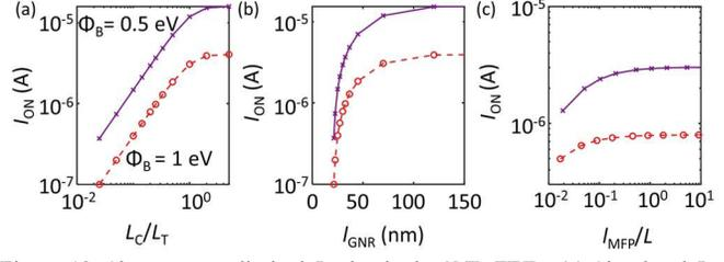
Figure 12. Short contact limited  $I_{ON}$  in single-GNR FETs. (a) Simulated  $I_{ON}$  versus  $L_C/L_T$  when  $\Phi_B$  is 0.5 eV (purple), and 1.0 eV (red). (b) Simulated  $I_{ON}$  versus  $l_{GNR}$  (c) Simulated  $I_{ON}$  versus  $l_{MFP}/L$ .  $V_{DS} = -1$  V,  $V_{GS} = -3$  V.
