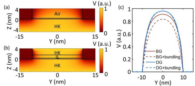
Figure 10. Numerical simulation of the electrostatics of BG and DG GNR transistors. (a) Potential mapping of the BG transistor. (b) Potential mapping of the DG transistor. (c) Potential along the GNR channel.
