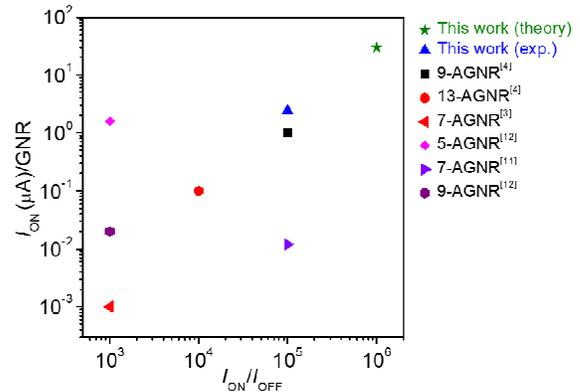
Figure 14. GNR FET devices benchmark. The maximum  $I_{ON}$  (per GNR) and  $I_{ON}/I_{OFF}$  ratio values are obtained from the devices fabricated with bottom-up synthesized 5-, 7-, 9- and 13-AGNRs at  $|V_{DS}| = 1$  V.
