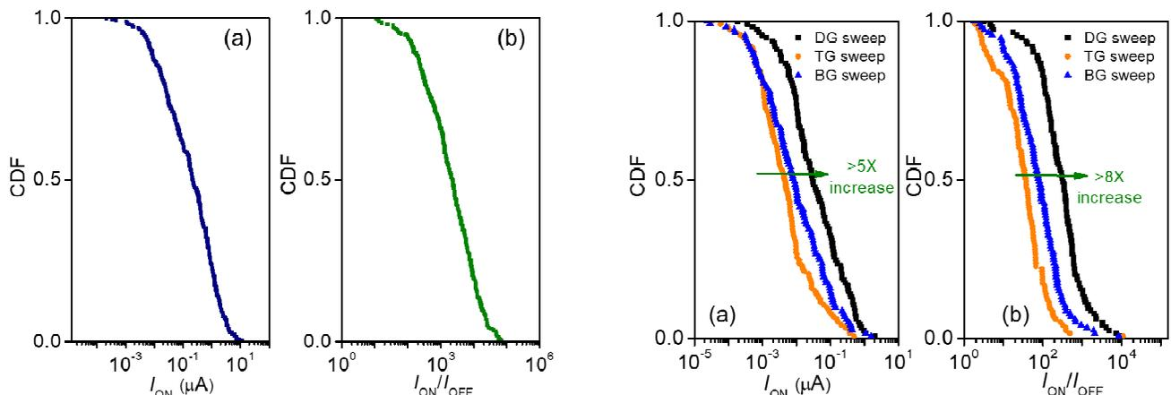
Figure 6. CDF of the  $I_{ON}$  (a) and the  $I_{ON}/I_{OFF}$  (b) in 113 DG FETs with BG ( $V_{BG} = 3 \text{ V}$  to  $-3 \text{ V}$ ,  $V_{TG} = 0$ ), TG ( $V_{TG} = 2 \text{ V}$  to  $-2 \text{ V}$ ,  $V_{BG} = 0$ ), and DG ( $V_{DG} = V_{BG} = V_{TG} = 2 \text{ V}$  to  $-2 \text{ V}$ ) sweeps.
