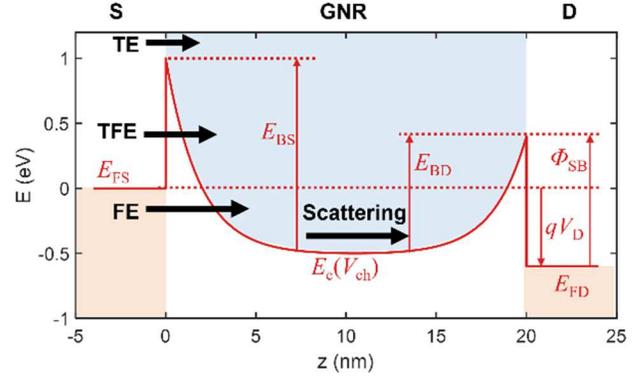
Figure 8. The energy band diagram along 9-AGNR channel. The thermionic emission (TE) current, the thermionic field emission (TFE) current, and the field emission (FE) current are considered at the SB; and the carrier scattering is considered in the GNR channel.
