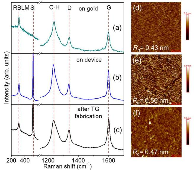
Figure 2. Raman spectra of the GNRs on gold (a), after transfer and device processing (b), and after TG dielectric deposition (c), collected with 785 nm wavelength laser excitation. AFM images ( $1 \times 1 \mu\text{m}$ ) of the local back gate (HfO<sub>2</sub>/W/SiO<sub>2</sub>/Si) before (d) and after (e) the GNR transfer, and after (f) TG dielectric deposition.
