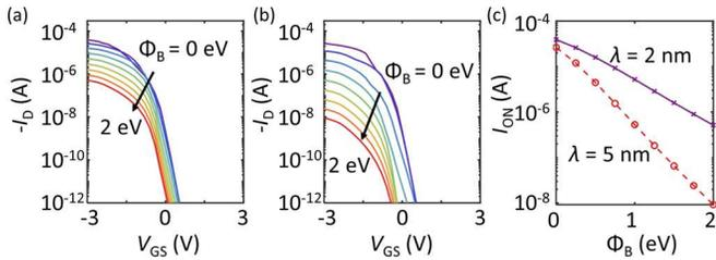
Figure 11. The effects of  $\Phi_B$  and  $\lambda$ . (a) simulated  $I_D$ - $V_{GS}$  characteristics with  $\lambda = 2$  nm,  $V_{DS} = -1$  V, and different  $\Phi_B$ . (b) simulated  $I_D$ - $V_{GS}$  characteristics with  $\lambda = 5$  nm,  $V_{DS} = -1$  V, and different  $\Phi_B$ . (c) simulated  $I_{ON}$  versus  $\Phi_B$  when  $\lambda$  is 2 nm (purple), and 5 nm (red).
