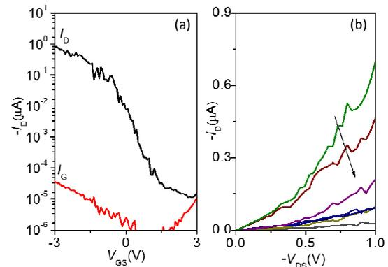
Figure 4.  $I_D$ - $V_{GS}$  (a) and  $I_D$ - $V_{DS}$  (with  $V_{GS}$  varying from  $-3 \text{ V}$  to  $3 \text{ V}$  with  $0.5 \text{ V}$  steps) (b) characteristics of a BG GNRFET. All device measurements are performed at  $V_{DS} = -1 \text{ V}$  under vacuum.
