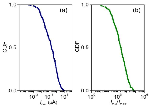
Figure 5. Cumulative distribution function (CDF) of the  $I_{ON}$  (a) and the  $I_{ON}/I_{OFF}$  (b) in 274 BG devices. The devices show an  $I_{ON}/I_{OFF}$  up to  $\sim 10^5$ , and an  $I_{ON}$  up to  $\sim 12 \mu\text{A}$  ( $2.4 \mu\text{A}/\text{GNR}$ ) for a device with  $L \sim 40 \text{ nm}$  and  $W = 200 \text{ nm}$  ( $\sim 5 \text{ GNRs}$  per the channel).
