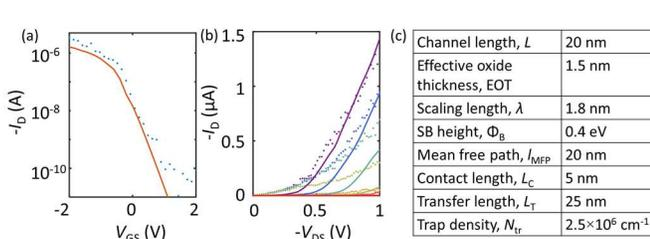
Figure 9. Experimental verification of the single 9-AGNR FET model. (a)  $I_D$ - $V_{GS}$  characteristics with  $V_{DS} = -1$  V. (b)  $I_D$ - $V_{DS}$  characteristics with  $V_{GS}$  varying from  $-1.8$  V to  $0.7$  V with  $0.5$  V steps. The solid lines are simulation results. The dots are experimental results. (c) Parameters used in the simulation that best matches the experimental results.
