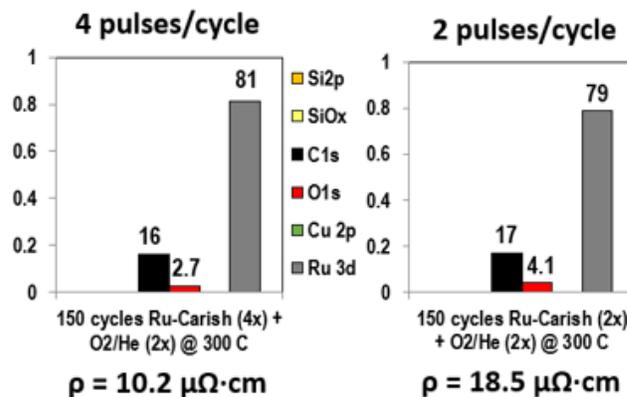
**Fig. 1. Effect of Ru-Carish pulses on Ru resistivity.** At 300 °C, after 150 cycles at 2 pulses per cycle of Ru-Carish, the film contains roughly 4.1% O, with a resistivity of 18.5  $\mu\Omega\cdot\text{cm}$ . Doubling the number of pulses reduces the percentage to 2.7%, with a decrease in resistivity to 10.2  $\mu\Omega\cdot\text{cm}$ .
