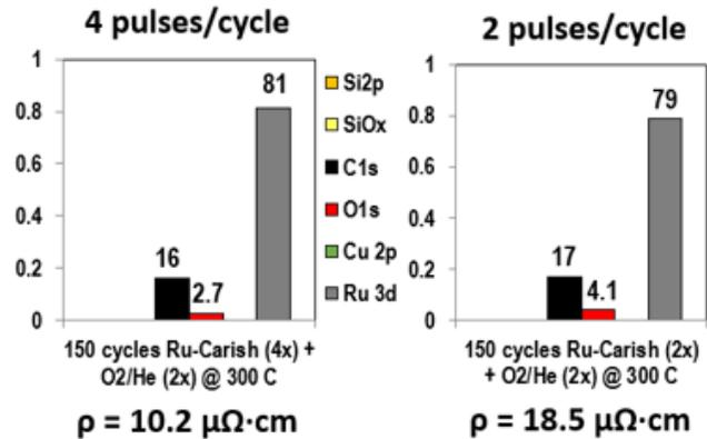
**Fig. 1. Effect of Ru-Carish pulses on Ru resistivity.** At 300 °C, after 150 cycles at 2 pulses per cycle of Ru-Carish, the film contains roughly 4.1% O, with a resistivity of 18.5  $\mu\Omega\cdot\text{cm}$ . Doubling the number of pulses reduces the percentage to 2.7%, with a decrease in resistivity to 10.2  $\mu\Omega\cdot\text{cm}$ .
