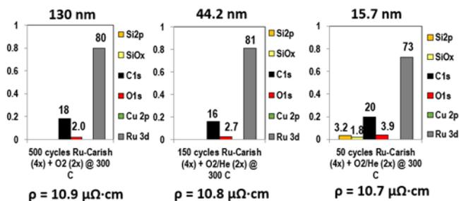
**Fig. 2. Resistivity-thickness relationship for Ru ALD.** At 300 °C and 4 pulses/cycle, the growth rate was determined to be 0.25 nm/cycle, with low oxygen persisting to 15.7 nm film thickness. Thickness measurement for the 130 nm film was performed via cross-sectional SEM, while thicknesses for the 44.2 and 15.7 nm films were determined via XRR. Four-point-probe resistance measurements showed resistivities of 10.9, 10.8, and 10.7  $\mu\Omega\cdot\text{cm}$ , respectively.
