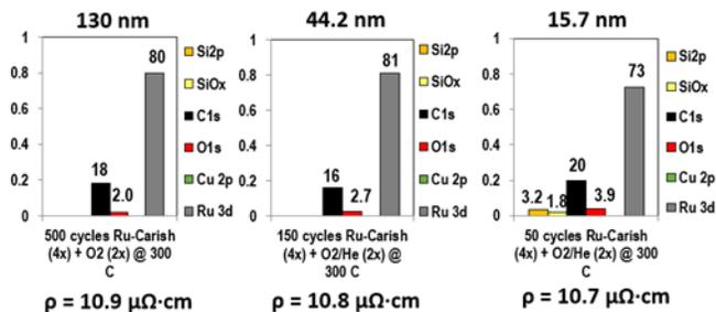
**Fig. 2. Resistivity-thickness relationship for Ru ALD.** At 300 °C and 4 pulses/cycle, the growth rate was determined to be 0.25 nm/cycle, with low oxygen persisting to 15.7 nm film thickness. Thickness measurement for the 130 nm film was performed via cross-sectional SEM, while thicknesses for the 44.2 and 15.7 nm films were determined via XRR. Four-point-probe resistance measurements showed resistivities of 10.9, 10.8, and 10.7  $\mu\Omega\cdot\text{cm}$ , respectively.
