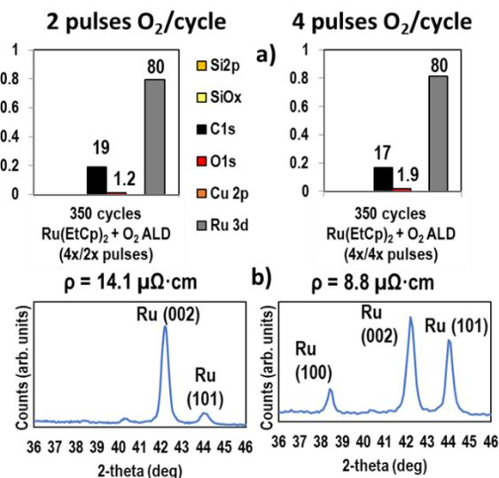
**Fig. 4. Resistivity-oxygen dose relationship for Ru ALD using Ru(EtCp)<sub>2</sub>.** At 2 pulses/cycle, growth rate was 0.9 Å/cycle, while at 4 pulses/cycle, growth rate was 1.0 Å/cycle. a) Oxygen content of both films was sub 2%, with the 2 pulse and 4 pulse/cycle films having a resistivity of 14.1 and 8.8  $\mu\Omega\cdot\text{cm}$ , respectively. b) XRD and XRR of the films show that the Ru(002) peak is dominant, but the Ru(101) grain size increases from 18.4 nm to 28.0 nm.
