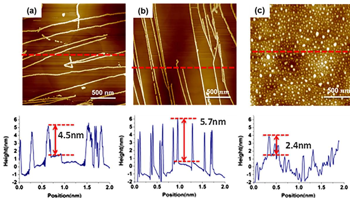
Fig. 1. AFM images of 50 cycles of  $\text{Al}_2\text{O}_3$  films on HOPG with different ALD temperatures. (a) 200 °C; the ridges along the step edges are 4.5 nm tall; (b) 150 °C; the ridges along the step edges are 5.7 nm tall; (c) 50 °C; the height and diameter of the particles are  $2 \pm 0.4$  nm and  $20 \pm 9.5$ . Each ALD cycle consisted of a 600 ms TMA pulse, a 500 ms Ar purge, a 50 ms  $\text{H}_2\text{O}$  pulse, and a 500 ms Ar purge.
