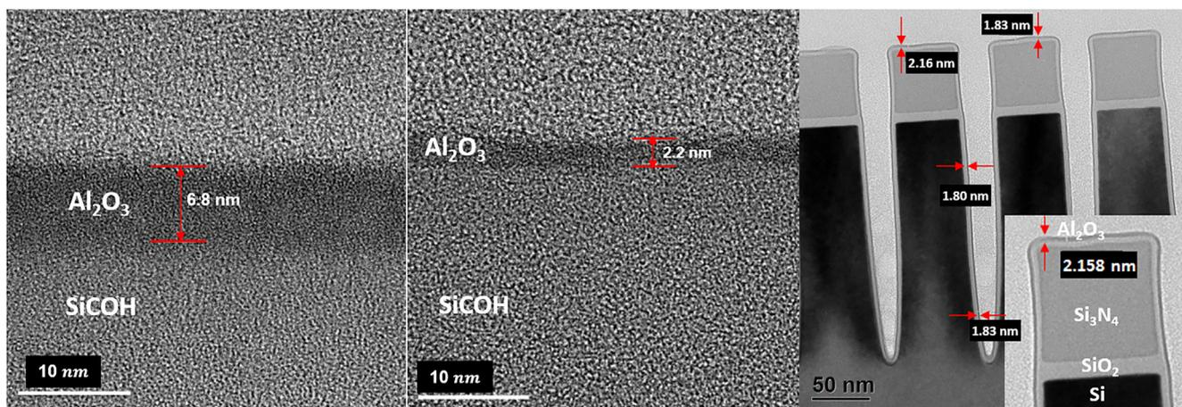
Fig. 4. (a), (b) TEM images of 50 cycles and 13 cycles of Al<sub>2</sub>O<sub>3</sub> ALD on hydrogenated silicon oxycarbide (H:SiOC) substrates. (c) TEM image of 20 cycles of Al<sub>2</sub>O<sub>3</sub> ALD on high aspect ratio Si<sub>3</sub>N<sub>4</sub>/SiO<sub>2</sub>/Si fin structures. The black outmost layer is Al<sub>2</sub>O<sub>3</sub>. The ALD cycles consisted of a 200 ms TMA pulse, a 10 s Ar purge, a 50 ms H<sub>2</sub>O pulse, and a 10 s Ar purge at 50 °C.
