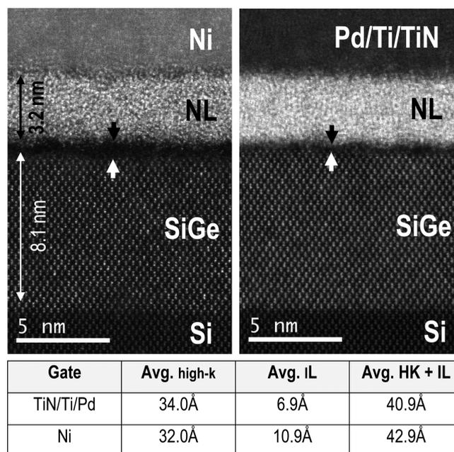
**Figure 8.** TEM analysis of interface thickness. HAADF images of Ni- and Pd/Ti/TiN-gated MOSCAP devices and table for average thickness of ILs and HfO<sub>2</sub>–Al<sub>2</sub>O<sub>3</sub> nanolaminate (NL) gate oxide. Ti-gated device shows thinner IL in comparison with the Ni control.
