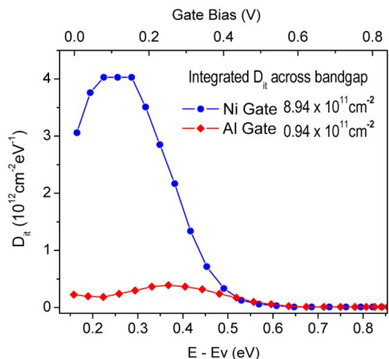
**Figure 3.** Interface defect density distributions for Al- and Ni-gated MOSCAP devices extracted with the full interface state model. In comparison with Ni controls, Al gettering gate devices show lower defect densities across the full energy range of the band gap. The integrated defect densities indicate a ~10× reduction in total defect density across the band gap with Al-gated device.
