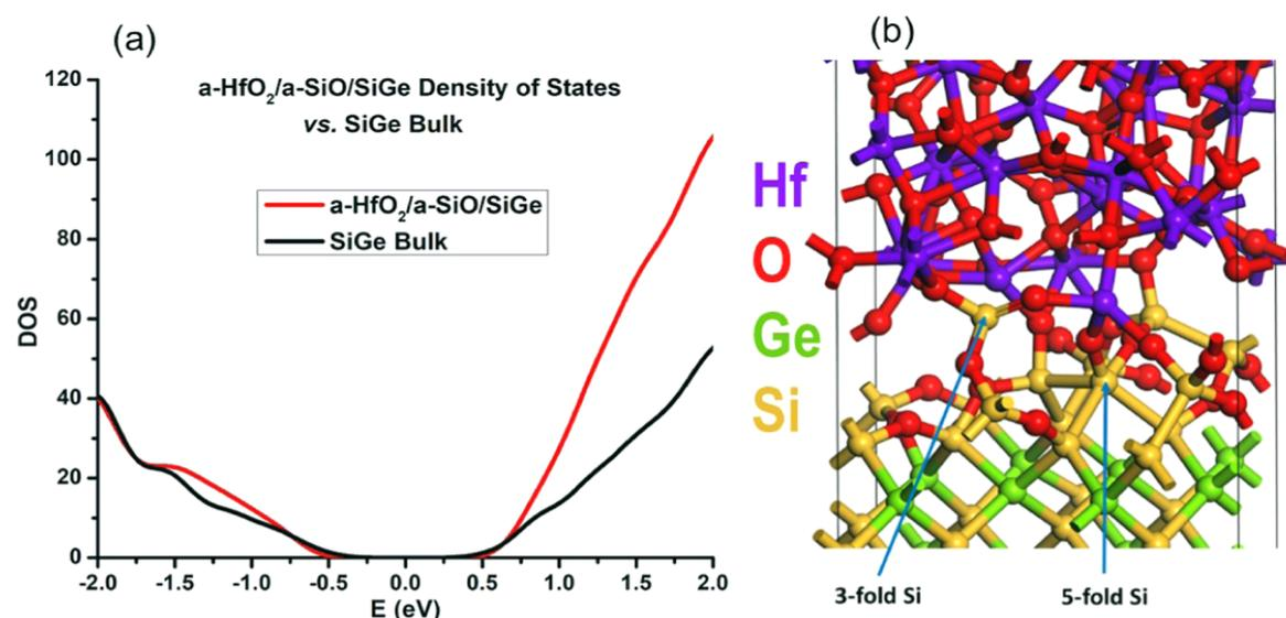
**Figure 6.** Density of states (a) and (b) interface bonding configuration for bulk SiGe and HfO<sub>2</sub>/SiO/SiGe. DFT results for annealed and relaxed a-HfO<sub>2</sub>/a-SiO/SiGe shows no energy states in band gap very similar to bulk SiGe. Corresponding interface structures illustrates 3-fold Si and 5-fold Si along with 4-fold Si bonding. Note the interfacial Si bonded to O, which is in nonstandard coordination, consistent with ionic bonding.
