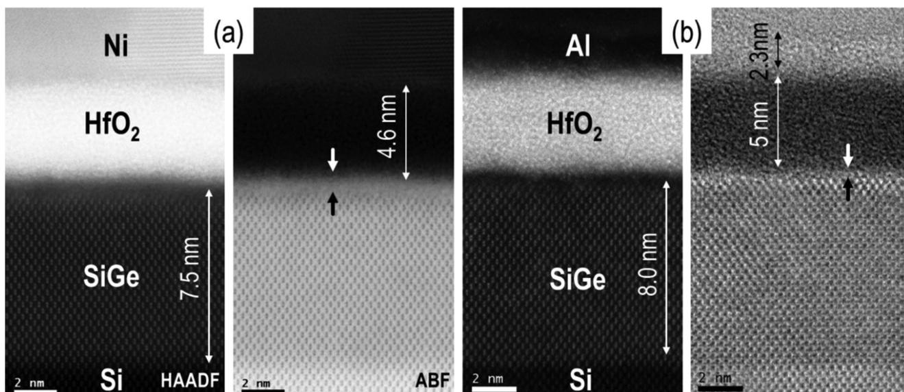
**Figure 4.** HR-STEM images of control Ni (a) and Al (b) gate  $\text{HfO}_2/\text{SiGe}$  MOSCAPs. In these images, oxide structures and regions defined according to contrast difference in which Ni-gated device displays two regions, gate oxide and IL, in contrast to Al, which has additional layer of 2.3 nm on gate oxide. In comparison to Ni control, the Al-gated device shows sub-0.5 nm interfacial oxide layer in various locations.
