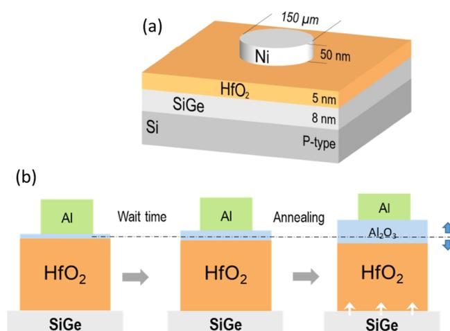
**Figure 1.** Schematic diagram of MOSCAP structure and gettering process. (a) Structure of the MOSCAP device. (b) Oxygen gettering process with an Al gettering gate. Al metal oxidizes with time and during forming gas anneal by the oxygen scavenged from interface as well as the excess of oxygen in  $\text{HfO}_2$ . White arrows denote scavenged oxygen from the interface during the anneal.
