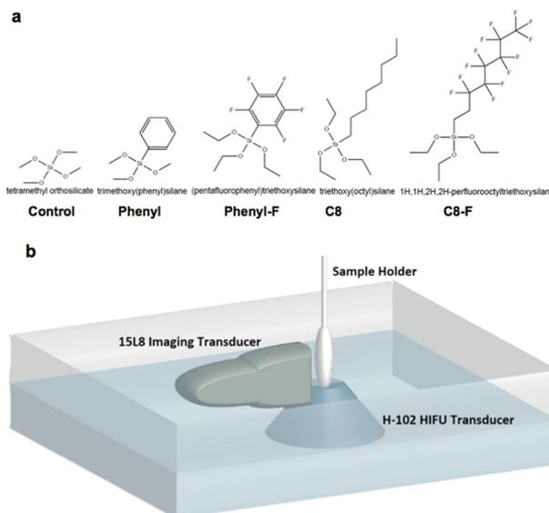
**Figure 1.** Structures of R-group-substituted trialkoxysilanes and experimental setup for ultrasound testing of nanoshells. A) Molecular structures and naming scheme of R-group-substituted trialkoxysilanes used in the modified sol–gel synthesis. B) Experimental setup for ultrasound testing of nanoshells. Nanoshells were suspended in the sample holder at 400 μg mL<sup>-1</sup>. The imaging transducer and the HIFU transducer were aligned orthogonally.
