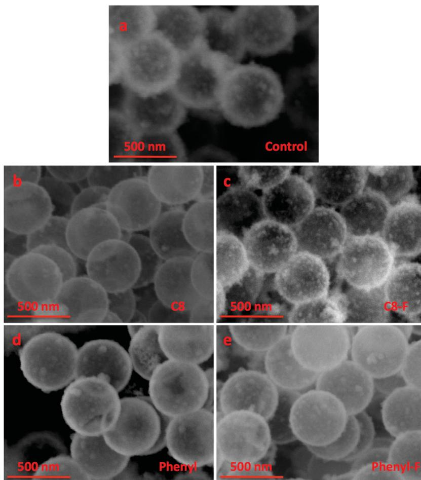
**Figure 2.** Scanning electron microscopy of various formulations at 74 K magnification after nanoshells have been calcined. A) Control nanoshells. B) Nanoshells synthesized with C8. C) Nanoshells synthesized with C8-F. D) Nanoshells synthesized with phenyl. E) Nanoshells synthesized with phenyl-F. The transparent images of the C8 and phenyl particles are consistent with the nanoflakes-forming shells of a few nanometer thickness.
