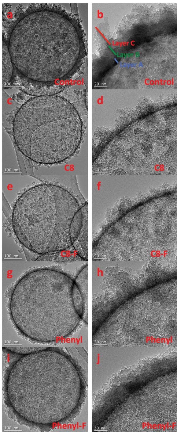
**Figure 6.** TEM images of all nanoshell formulations. All images were taken at 40 000 $\times$  magnification and then 150 000 $\times$  magnification for high-resolution images of the shells. A,B) **Control** nanoshells. C,D) Nanoshells synthesized with **C8**. E,F) Nanoshells synthesized with **C8-F**. G,H) Nanoshells synthesized with **phenyl**. I,J) Nanoshells synthesized with **phenyl-F**. The nanoshells synthesized with **C8** and **phenyl** had the thinnest walls.
