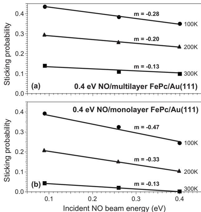
FIG. 3. Plot of NO sticking probability as a function of beam energy at 100, 200, and 300 K for the (a) ordered multilayer FePc and (b) ordered monolayer FePc films. All linear fits have a regression coefficient,  $R^2$ , greater than 0.95.
