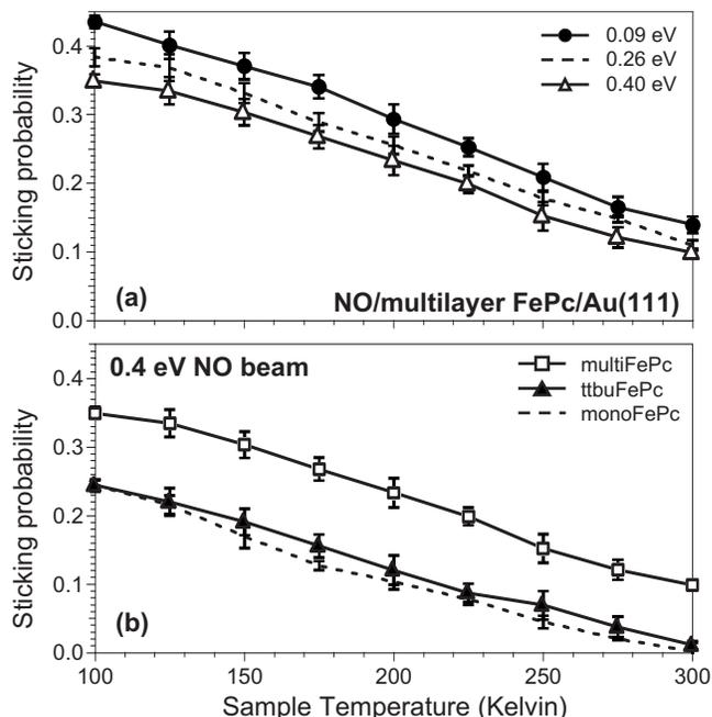
FIG. 2. Plot of NO sticking probabilities as a function of sample temperature at (a) varying NO beam energies (0.09 eV=filled circles, 0.26 eV=dashed line, and 0.40 eV=open triangles) for the multilayer FePc film and (b) 0.4 eV NO beam for the multilayer FePc (open squares), multilayer ttbu-FePc (filled triangles), and monolayer FePc (dashed line) films. All error bars shown are for the standard error of eight measurements at each temperature.
