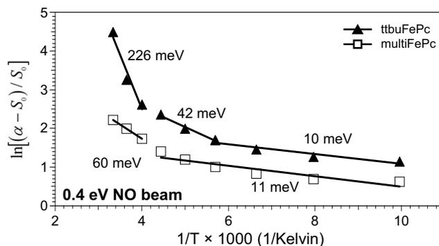
FIG. 5. Arrhenius plots for the 0.4 eV NO beam for the multilayer FePc (open squares) and multilayer ttbu-FePc (filled triangles) films. The monolayer FePc data were not shown as the results were nearly identical to the ttbu-FePc results.
