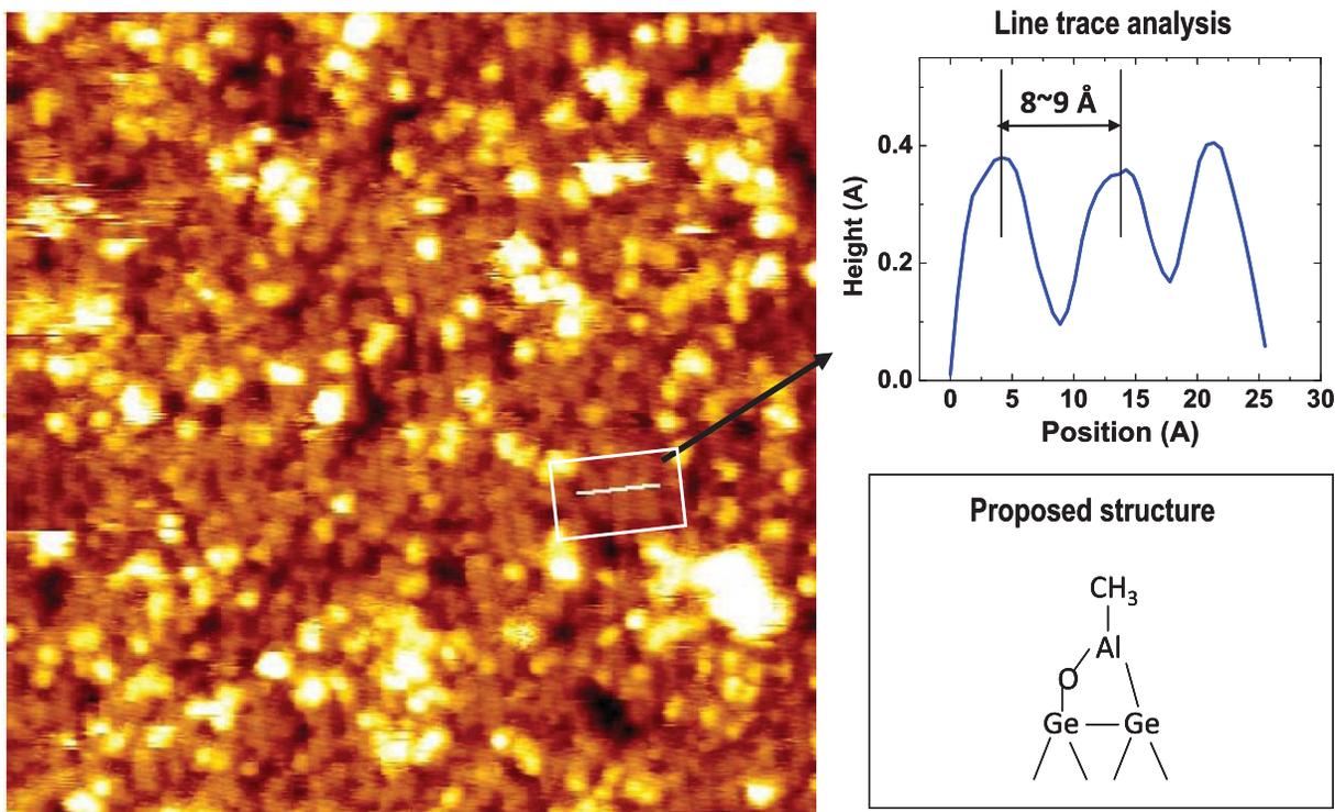
FIG. 4. Filled state STM image (30 nm × 30 nm) of  $7 \times 10^5$  L H<sub>2</sub>O dosed Ge(100) followed by 35 000 L TMA dosing at RT and annealing at 200 °C. An ordered structure is observed (white box). Line profile shows the spacing of vertical rows is ~9 Å and proposed structure is shown on the bottom right.
