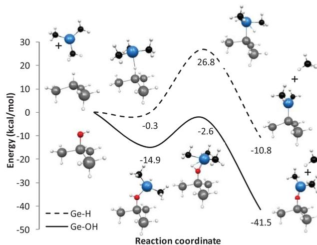
FIG. 6. Potential energy of surfaces calculated for the adsorption of TMA on -Ge-OH and -Ge-H. The stable and transition state structures for the TMA reactions are indicated. In these structures, the Ge atoms are displayed in grey, H in white, Al in blue, and O in red. The energies in kcal/mol were calculated relative to the energy of the reagents.
